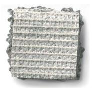
This is the last step of the process, when our secondary backing system is attached to the tufted primary by using a thin, smoothed layer of latex between the two backing systems.
